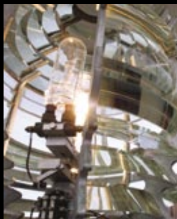
Light shines through the Fresnel lens inside Pemaquid Point Light in Bristol.
